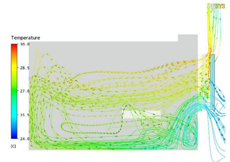
Arups CFD analysis showing a vertical section through the room. Air movement vectors (arrows) through room coloured by temperature.
