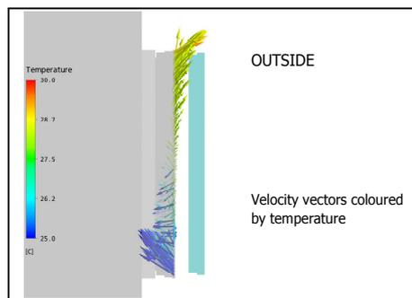
Arups CFD analysis showing a side view of air movement through an open parallel window with a flow rate in of 0.124m<sup>3</sup>/s (124 litres/s) & 10.9 air changes per hour
